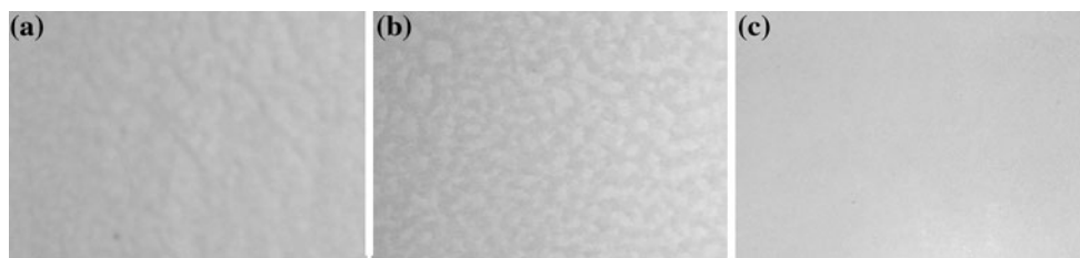
Fig. 2 Cast dispersions of MFC and PVA solution after at least 2 h under ambient conditions. The MFC load in all of the dispersions is 1%. The PVA solution concentrations are: a 1 %; b 2 % c 4 %
